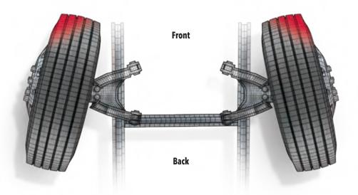
The distance between the front of the tires is less than the distance between the **TOE-IN** rear of the tires.
