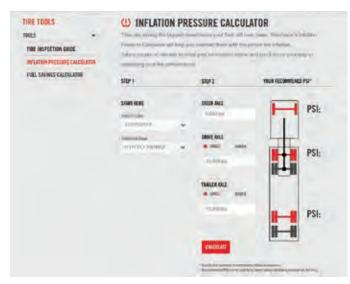
\* Results are minimum recommended inflation pressures. Recommended PSI are for cold tires; never adjust inflation pressures for hot tires.
