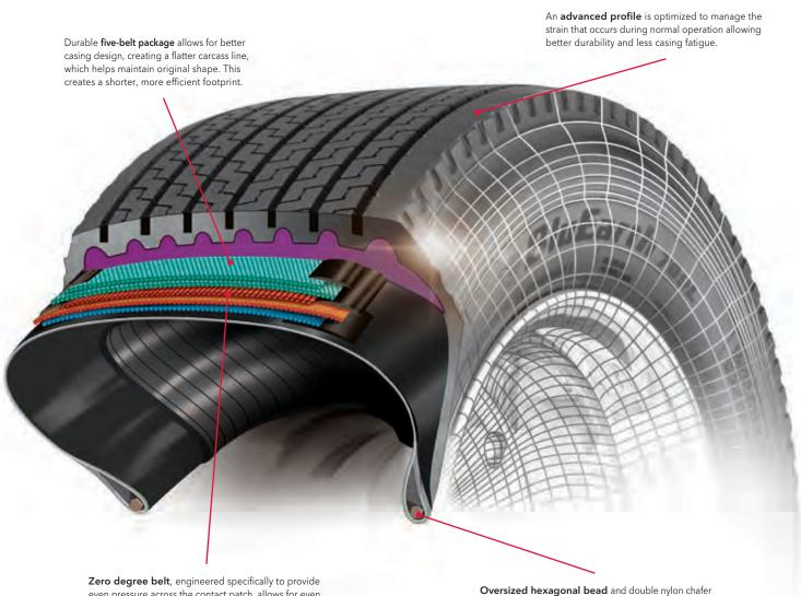
even pressure across the contact patch, allows for even weight distribution and vastly increased treadlife. **Oversized hexagonal bead** and double nylon chafer allow for easier mounting and provide even pressure along the wheel's circumference to reduce strain and increase the life of the tire.
