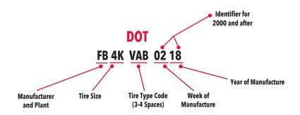
Some manufacturers place an additional code with a specific serial which identifies the specific tire model (a tire type code). This optional number is located on the sidewall opposite the DOT number.
